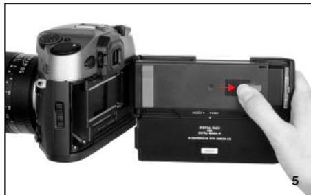
7. slide the protective cover (Ca) to the right (approx. 5 mm, Figure 6) and carefully remove it vertically from the rear panel.
