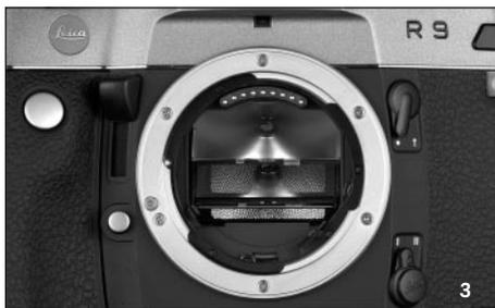
4. Then grip the tab on the focusing screen with the tweezers (front right).
