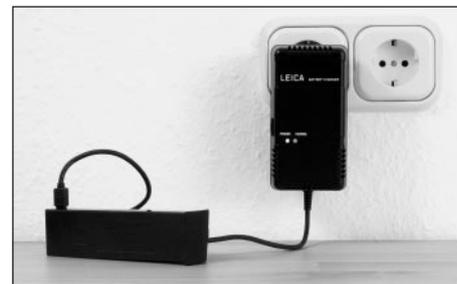
After charging is complete – approx. 2 hours<sup>1</sup> – the red LED goes out and the charging current is disconnected. There is therefore no risk of overcharging. Nevertheless, the charger should then be disconnected from the mains.
