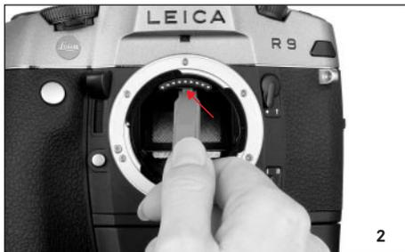
**Important:** To change the focusing screen, only use the tweezers; do not attempt to use your bare hands and ensure that you do not touch the focusing screen or the mirror with the tweezers or your hand while inserting, to prevent dirt and scratches on the sensitive surfaces.
