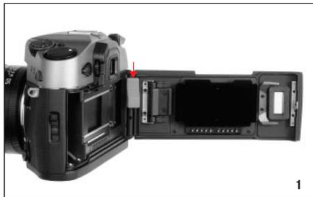
3. Press the slider and thus the moving upper joint pin on the back downwards. The back is thus unlocked and can be
